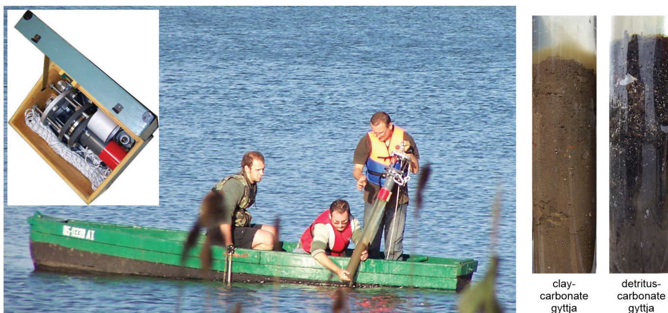
Figure 4. Collection of Gopło bottom sediments by sampler, and sample sediment cores.
